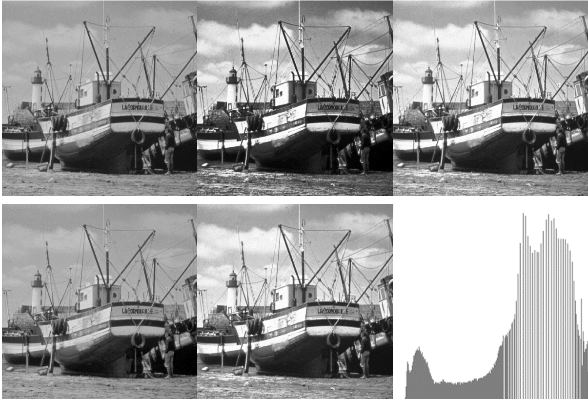
Figure 5. Ship: From top to bottom and left to right, the input image, WHE, MAX, LSHE, RSHE and histogram when reaching the maximum contrast value 0.607158 at the range [139:255].
