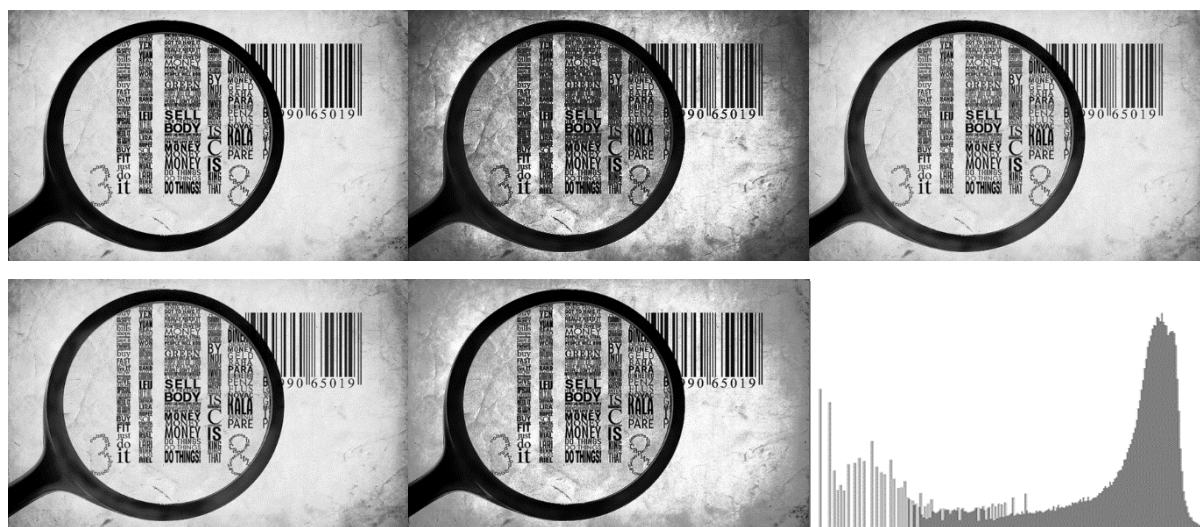
Figure 4. Magnifier: From top to bottom and left to right, the input image, WHE, MAX, LSHE, RSHE and histogram when reaching the maximum contrast value 0.666864 at the range [0:150].
