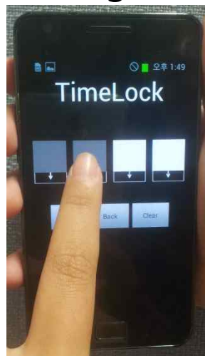
The user is entering the second digit by touching the appropriate button and counting the beeps or vibrations.
